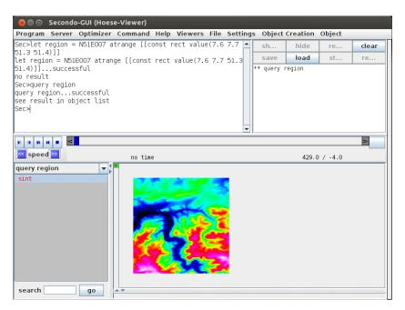
The slope must be calculated for the area of interest. Because x- and y-coordinates are given in degree and the height is given in meter the z-factor must be set to 111200.0. let region\_slope = region\_slope[111120.0]
